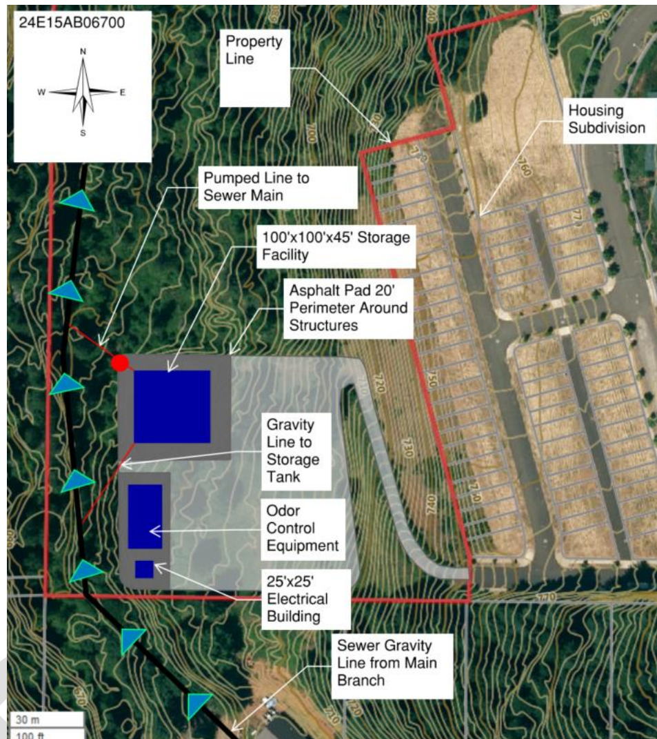
Figure 10-9: Collection System Storage Tank Location
